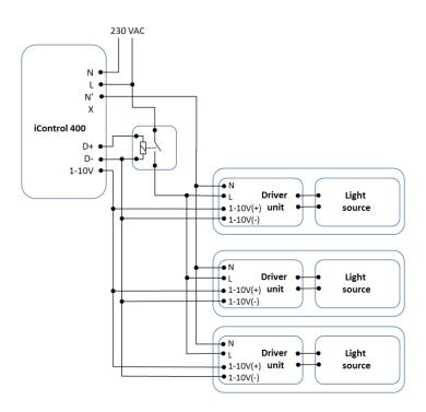
Note: Power supply is not routed through control unit, when energy consumption measurement is not used.
