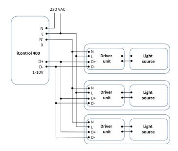
Note: Power supply is not routed through control unit, when energy consumption measurement is not used.
